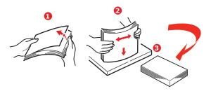
Load paper long edge feed (LEF) (letter headed paper face down and top edge towards the right of the printer) (1) up to mark (a)..
